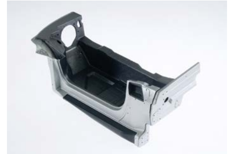
These 1/6 scale FDM prototypes helped Lamborghini Lab determine fit and improve load paths.
