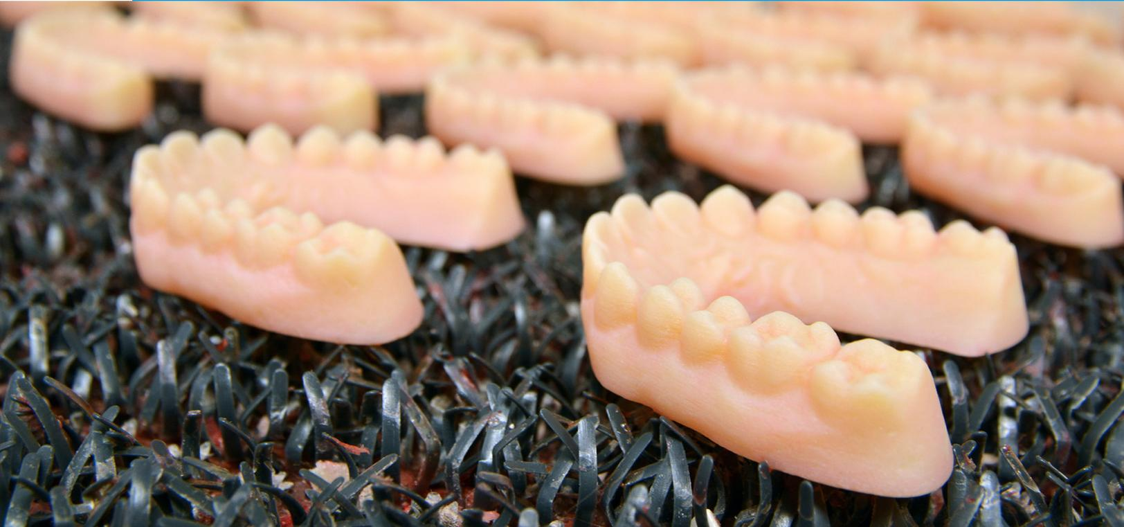
An array of clear aligner arches 3D printed on the Stratasys J700.
